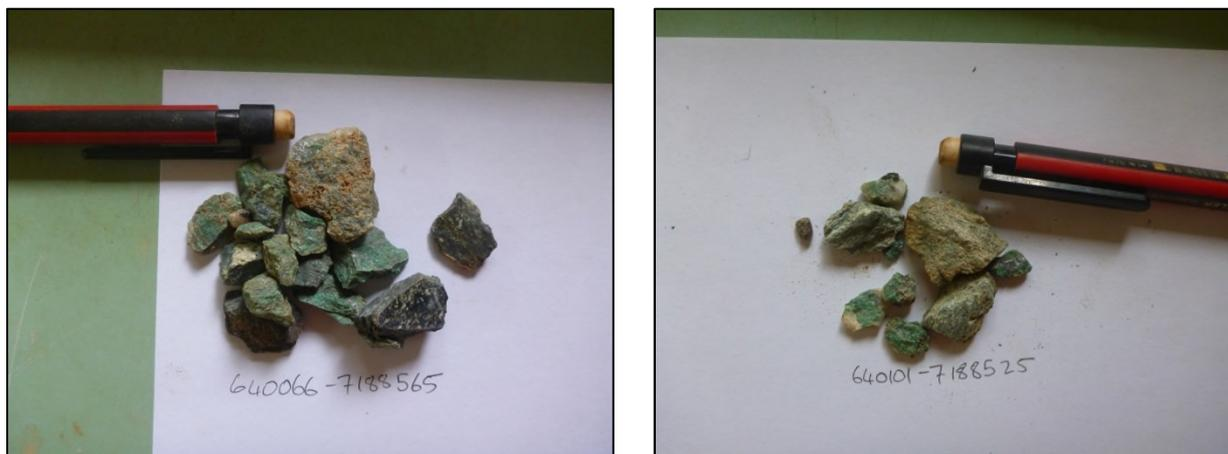
Figure 2: Malachite rich rock chip samples from RAB drilling
