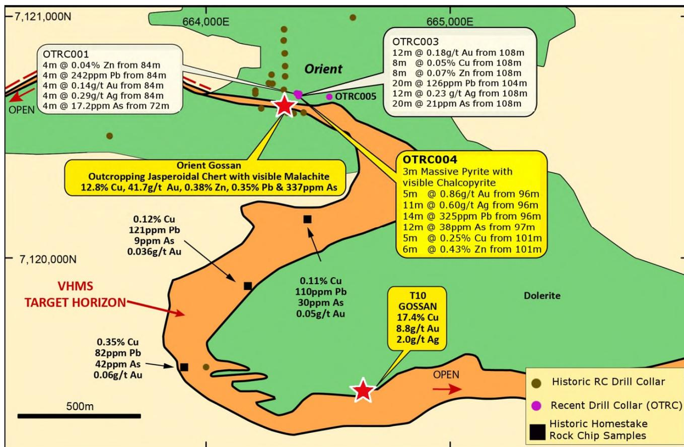
Figure 2: Orient – T10 prospective VHMS horizon
